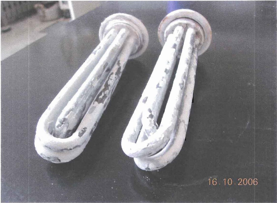
photo 4: electric heating pipe
