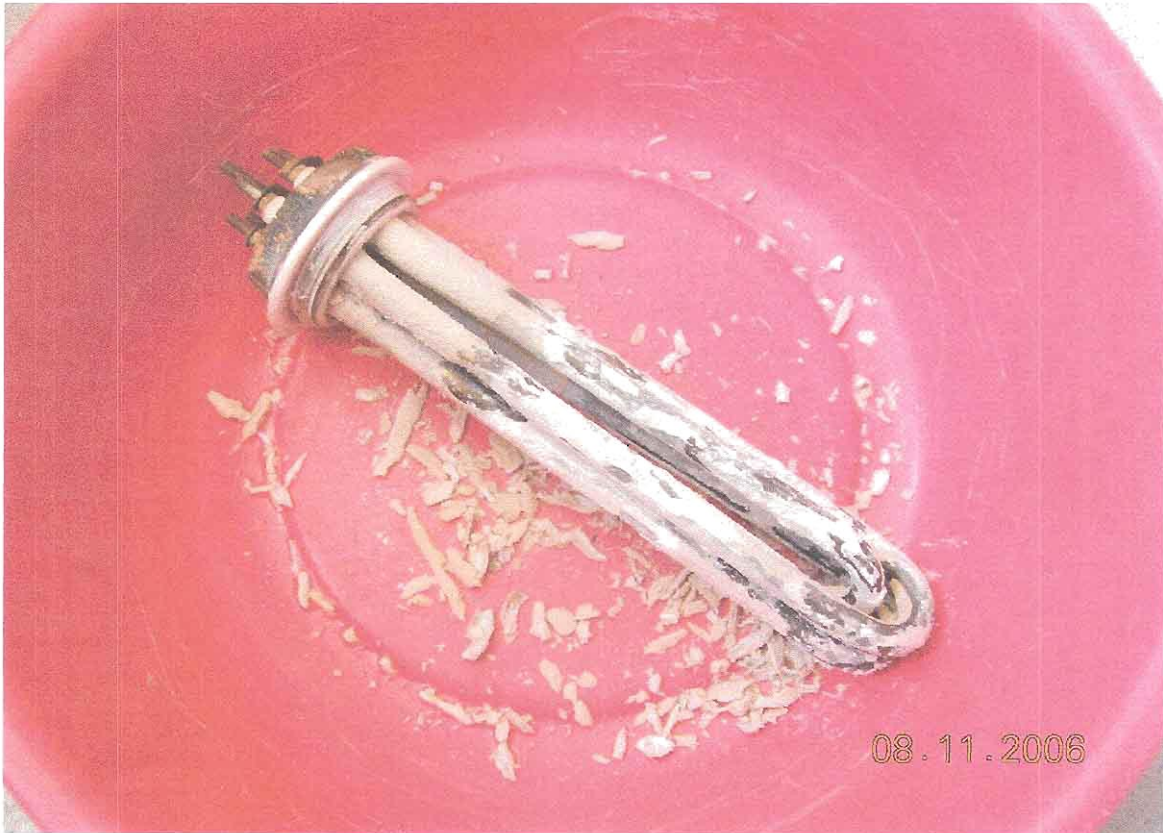
photo 2: the scale on the heating pipe become easy to be peeling off
